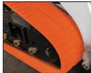
Optional non-marking multi-bar lug rubber tracks won't leave black rubber marks on hard surfaces like concrete.
