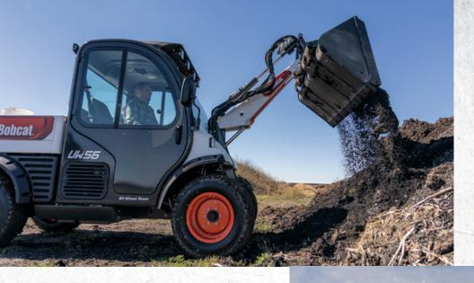
Toolcat utility work machines offer over 6½ feet of lift height for loading or placing materials.
